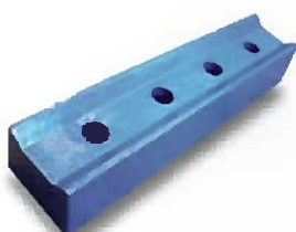
HAMMER MILL 8H IV MAT : SCMNM3 WEIGHT : 48 KGS.
