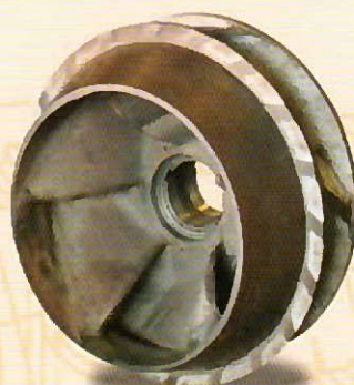
IMPELLER Size 938 mm, MAT : BS4844 GRADE 3D WEIGHT : 610 KGS.
