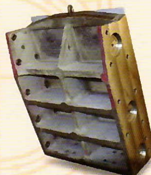
FRONT END FRAME MAT : AS2074/L1A WEIGHT : 2250 KGS.
