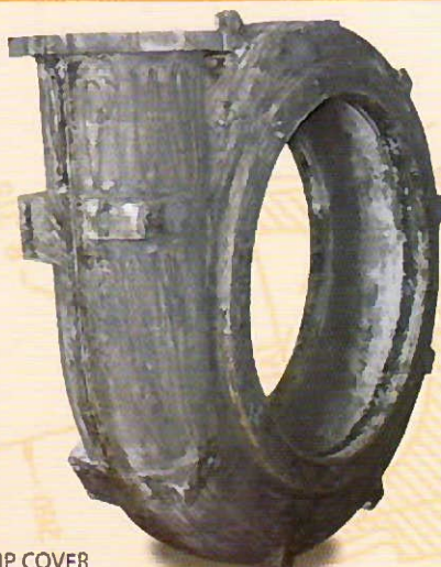
PUMP COVER MAT : GX 170 CrMo 25 2 WEIGHT : 4500 KGS.
